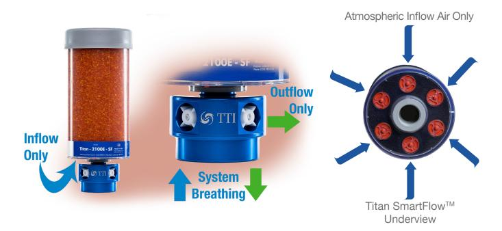
\* Titan SmartFlow™ PowerBreather™s (Titan-XXXX-SF) consist of all check valves positioned inward to exclusively inhale from the atmosphere, therefore must be used with the Titan-SF-A1 (1" FNPT) or Titan-SF-A2 (2" FNPT) SmartFlow™ Adapters to exhale all air out of the system.
