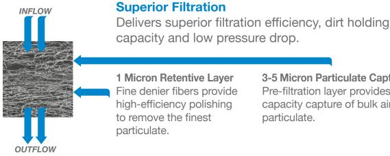
3-5 Micron Particulate Capture Layer Pre-filtration layer provides highcapacity capture of bulk airborne particulate.
